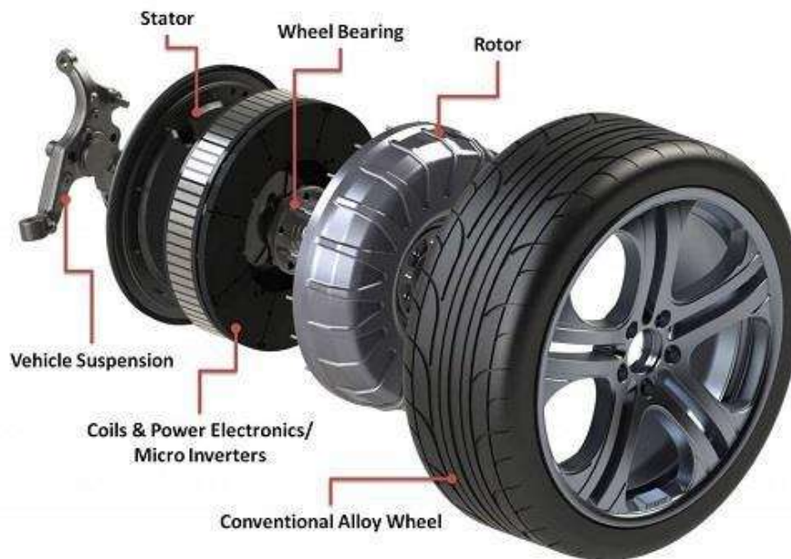
Fig4.4 : In wheel motor assembly
