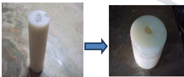
Fig.2. Reducing nylon diameter and drilling a hole
