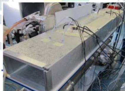
Fig 11: Inlet channel and sensors
