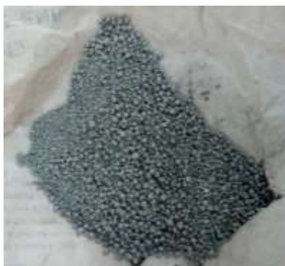
Improper cleaning of vail result in formation of intermediate compound
