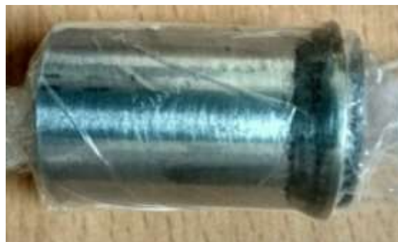
Loss of die shank material while compacting 15% siO 2 composite powder.
