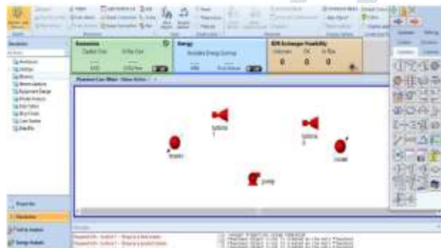
Fig:5.1-Adding components in flow sheet
