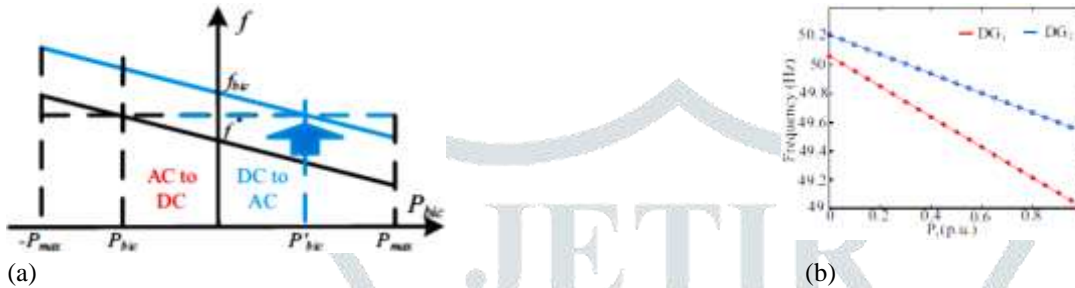
Figure 5: (a) Shifting Capability of BIC frequency power droop characteristic (b) Frequency Droop Characteristic
