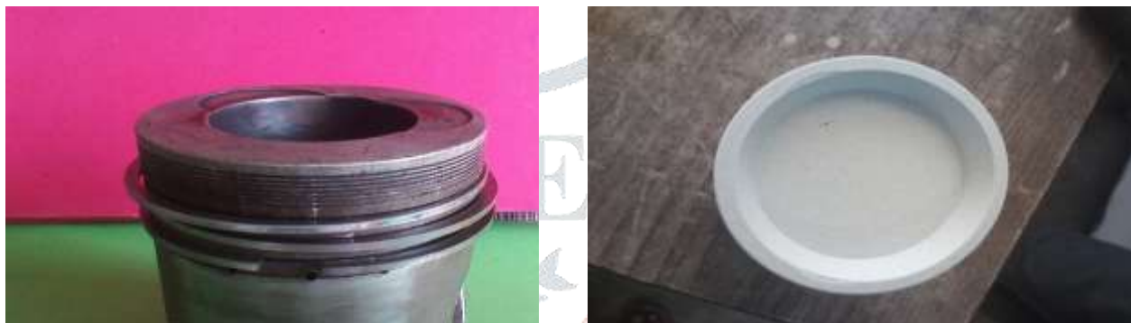
Fig.1. Shows snapshots of two different pistons i.e., Hemispherical bowl (left), CYSZ Coated bathtub piston (Right)
