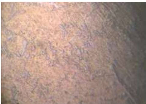
(a) As Received LM25 alloy at 450X
