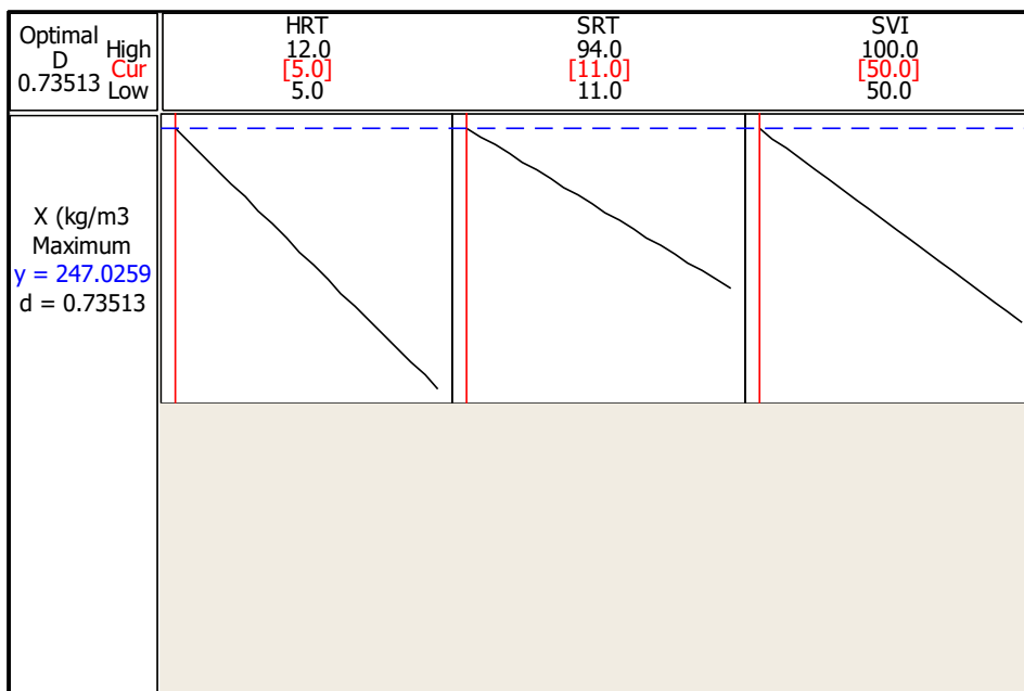
Figure 4 Desirability Plot to find the optimal levels in order to achieve maximum biomass production
