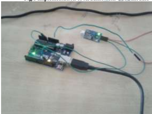
Fig.9 Implementation of Arduino with IR sensor
