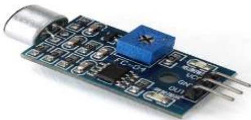
Fig.4 Schematic view of Sound sensor
