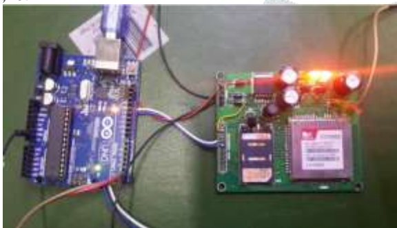
Fig.8 Implementation of Arduino with GSM module
