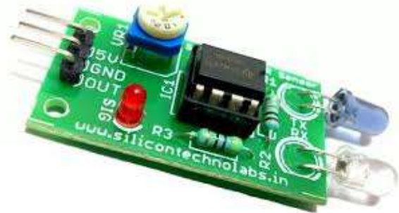
Fig.6 Schematic view of IR SENSOR
