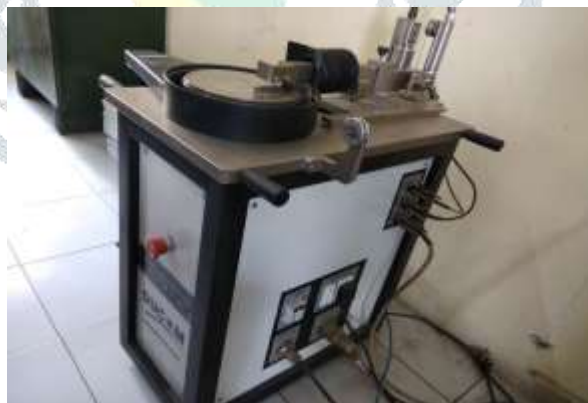
Fig 1. Pin on disc apparatus for the wear test
