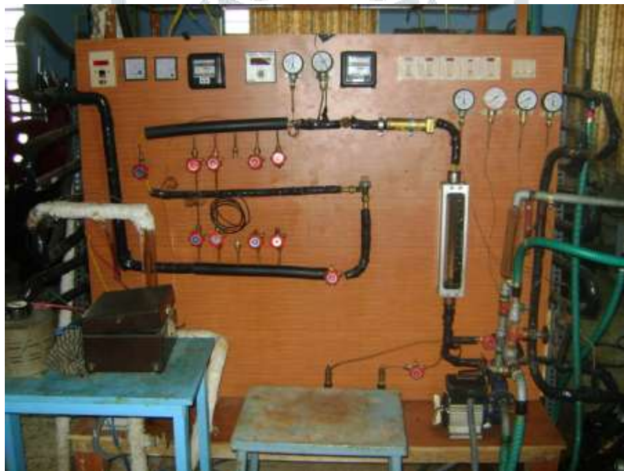
Figure 2 Experimental set-up used to test the performance of refrigerants
