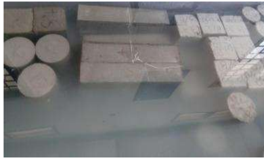
Fig 3 Curing of concrete
