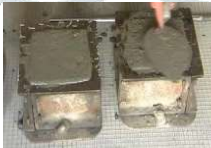
Fig 2 Casting of concrete
