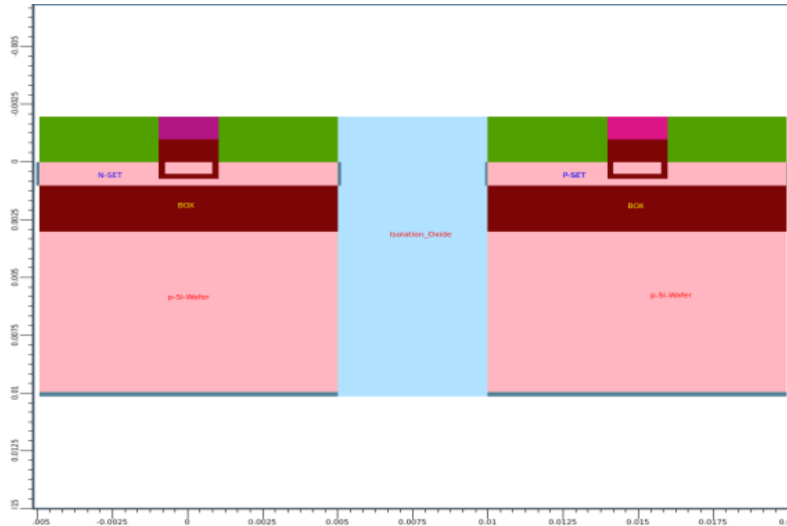
Figure 2.1 2-D view of inverter
