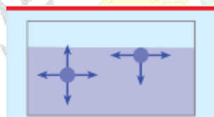
Fig 1: Model of the forces of cohesion acting on an internal molecule and surface molecule.
