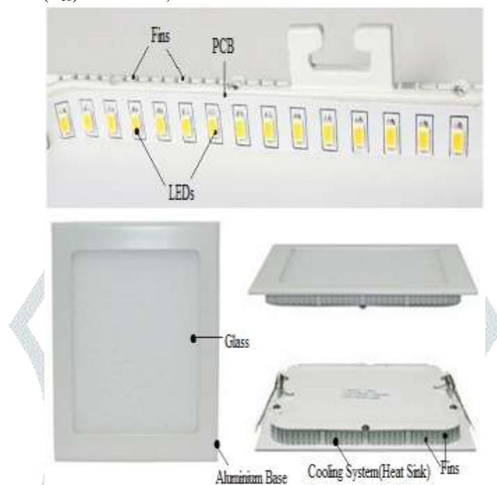
Figure 3: Schematic diagram of the 15W LED panel
