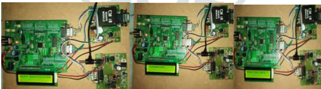
Fig.1 Wi-Fi Initializing, connection to server and access to authentication cards
