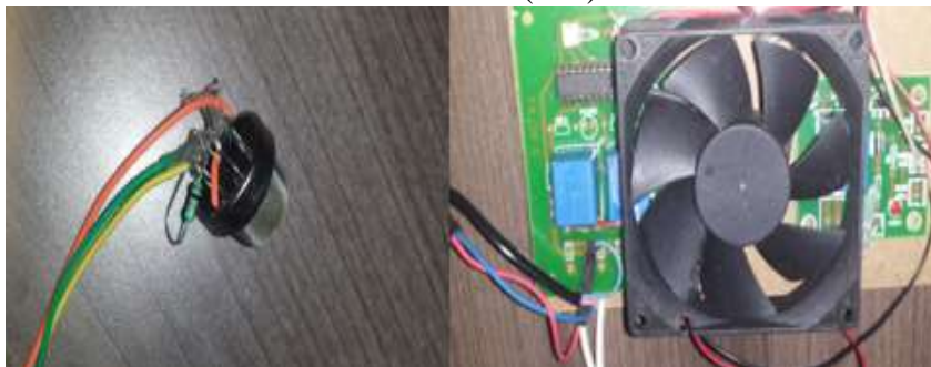
Fig2:MQ2 Gas sensor and Exhaust Fan
