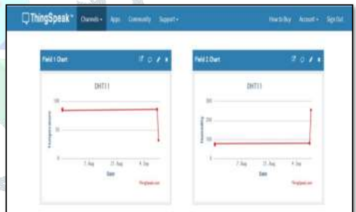
Fig.4.3(c) Temperature and humidity data from DHT 11 sensor on Thing speak
