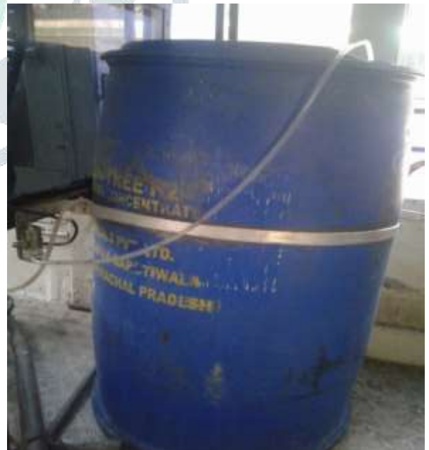
fig.4.2.210L.plastic drum in fitted inbus .
