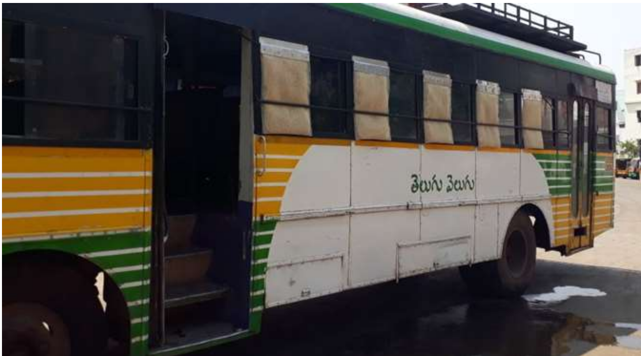
4.6. cooling pads arranged on bus left side as shown figure
