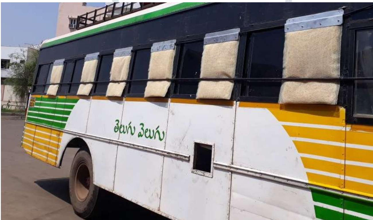
4.5.cooling pads arranged on bus right side as shown figure
