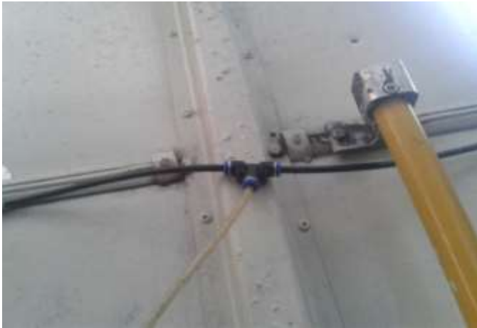
Fig4.3.T-connector and pipes fitted on inside top of the bus
