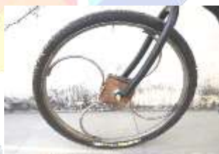
fig.2.2 Integral suspension wheel assembly
