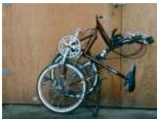
fig.2.1 Mid-frame horizontal folded frame
