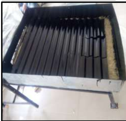
Fig: Flat Plate Collector
