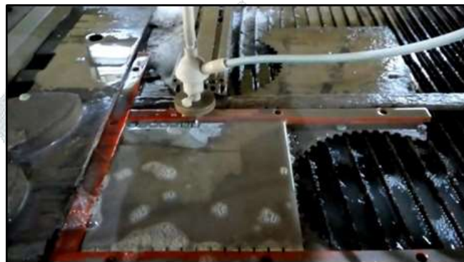
Fig.2.1. Inconel 601 during AWJM machining
