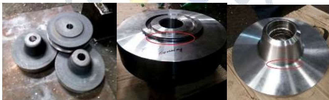
Figure 8: Unfilling defect at job
