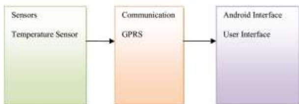
Fig. 1.1 Architecture of Remote Temperature Monitoring Application
