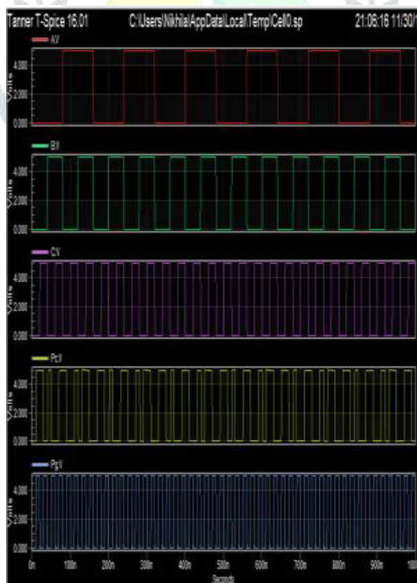
Figure.10: Even parity checker circuit Simulation Result
