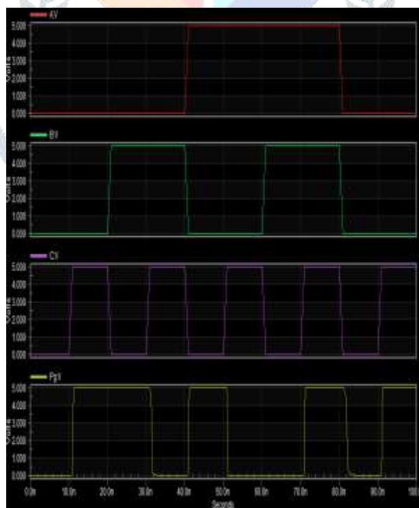
Figure.8: Even parity generator circuit Simulation Result
