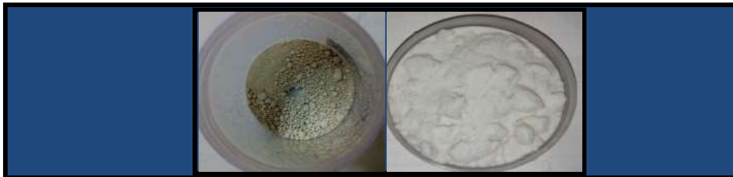
Fig1: Digital images of (a) Nano titanium particles and (b) Nano zinc particles
