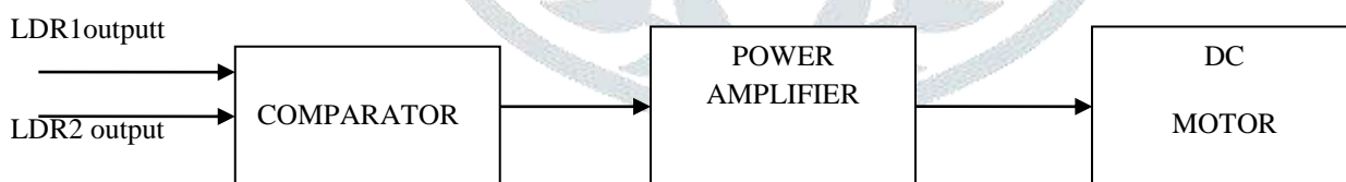
Fig.5: Block diagram of solar Tracking system
