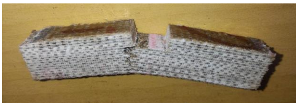
Fig.2.5 Specimen after Impact Test and Moisture absorption setup
