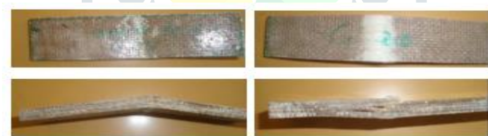
Fig. 2.4 Failed specimens after bending test
