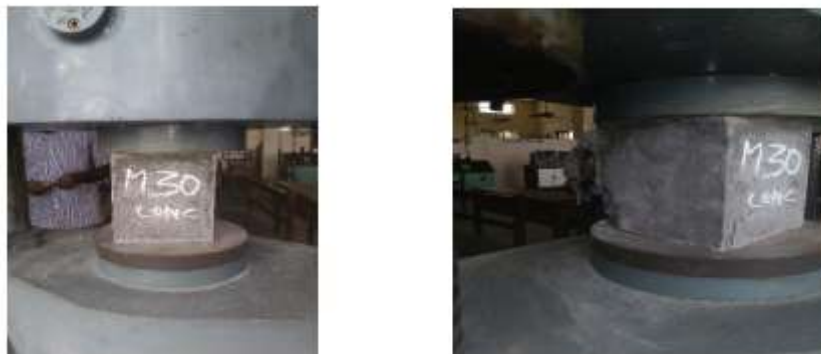
Fig 10: Testing of AAC Cube
