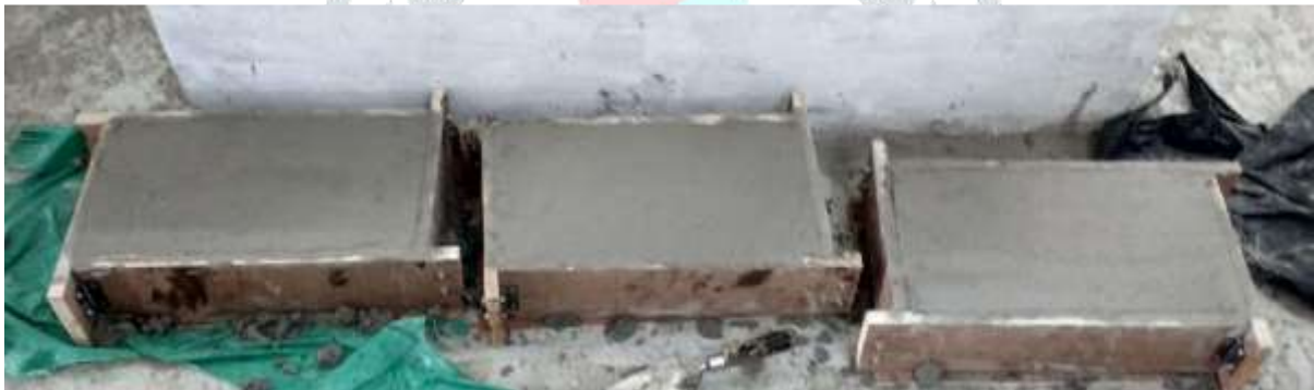
Fig 7:Finished Product of AAC Block
