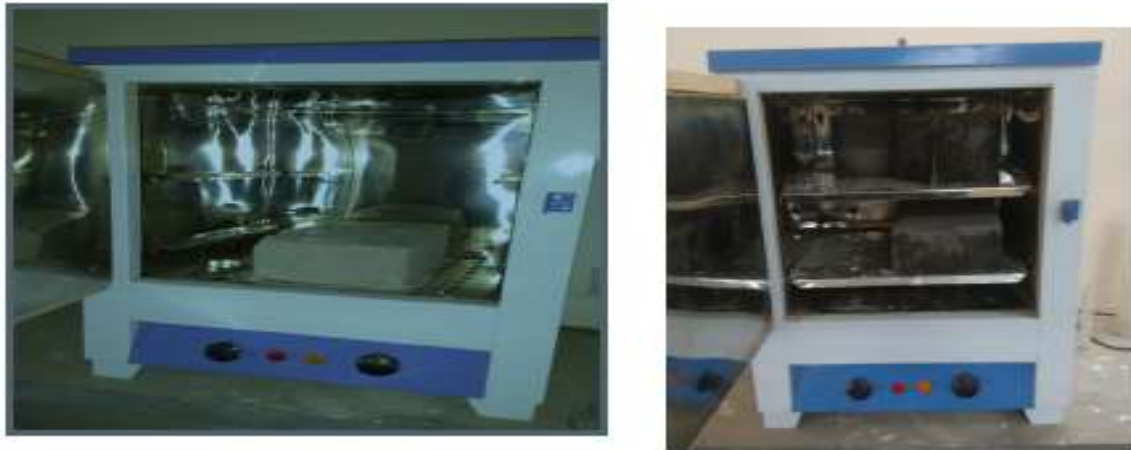
Fig 9: Heating of AAC Cube and Block
