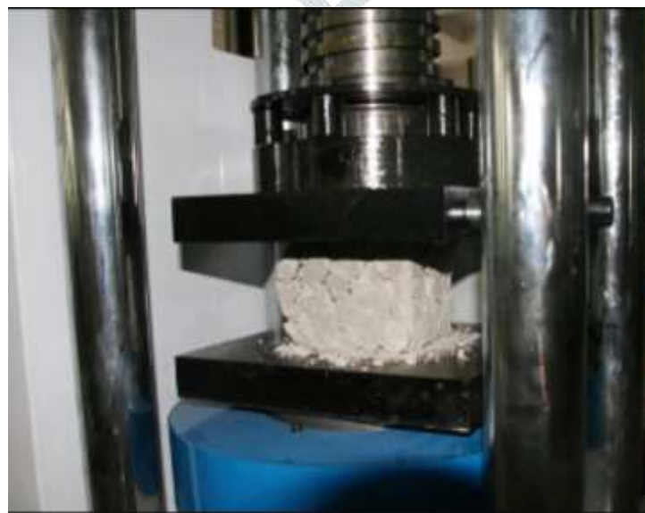
Fig 10: Testing of AAC Cube
