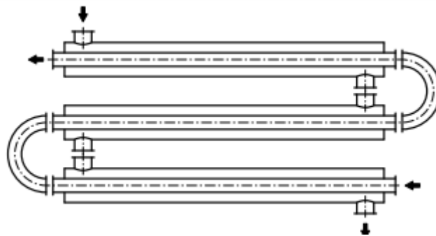
Figure 1.1: Countercurrent double-pipe heat exchanger
