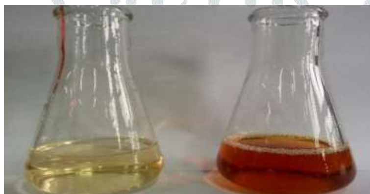
Fig. 2.2 (A) (B) 1 mM \text{AgNO}_3 without \text{C.papaya} extract 1mM \text{AgNO}_3 with C.papaya extract after 10 hrs of incubation
