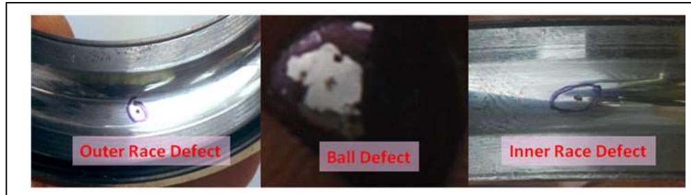
Fig.2. Seeded Localized defect on elements of ball bearing
