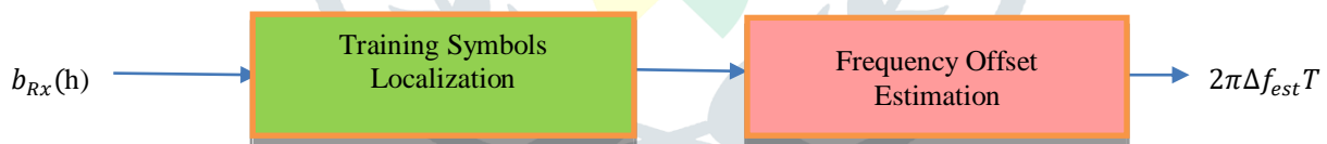
Figure: 9 Block Diagram of Training symbols and (FOE)Frequency Offset Estimation.[3]
