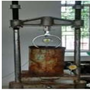
Fig. 4 Testing of Stone column
