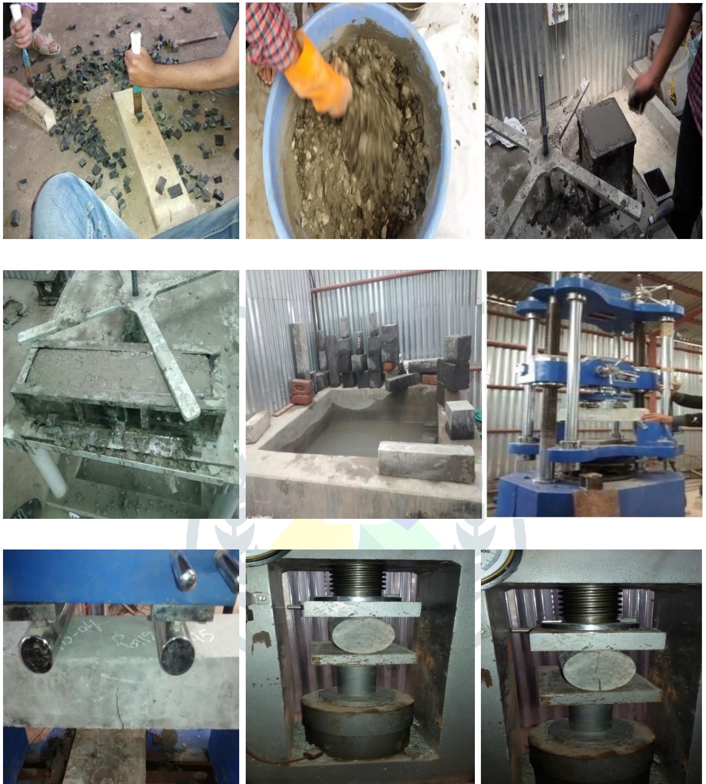
Fig 3.1: Different Stages of the Project- Manual Shredding of Tyre Rubber, Mixing of Concrete, Casting and Compaction of Samples, Curing and Testing of the Specimens.
