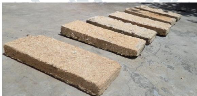
Fig.1. Sawdust Tiles developed for thermal insulation
