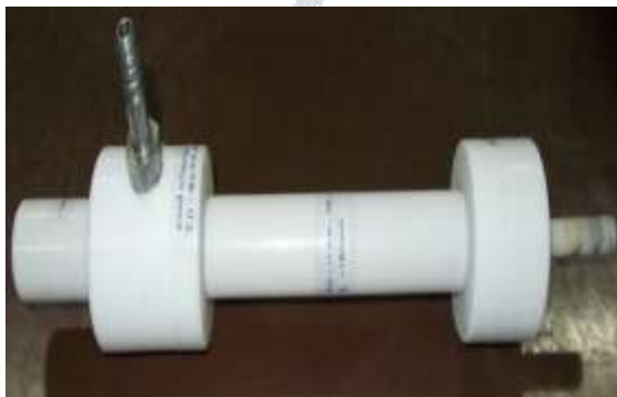
figure :2.vortex tube with PTFE Teflon material.
