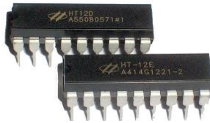
Figure 7. Encoder &amp; Decoder
