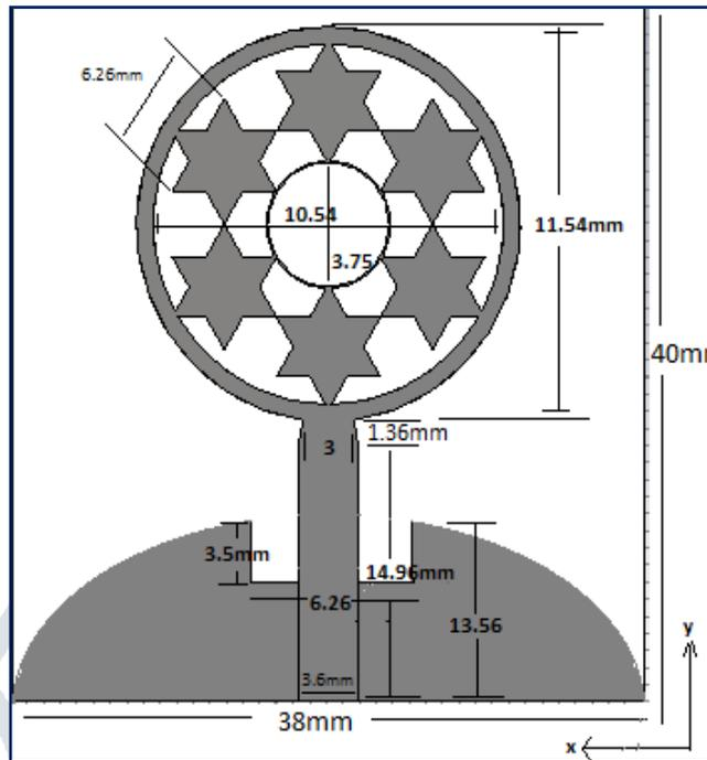
Figure 1: Geometry of the designed antenna
