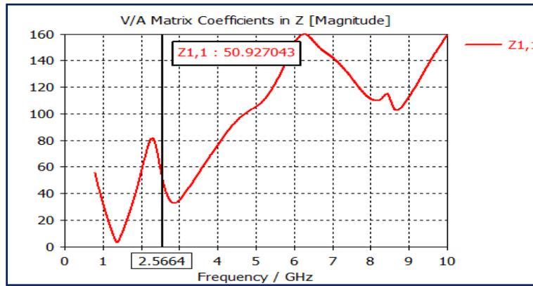
Figure 5: Impedance of fractal antenna
