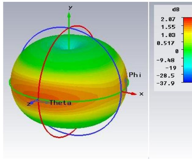
**Figure 7:** 3D radiation pattern of fractal antenna
