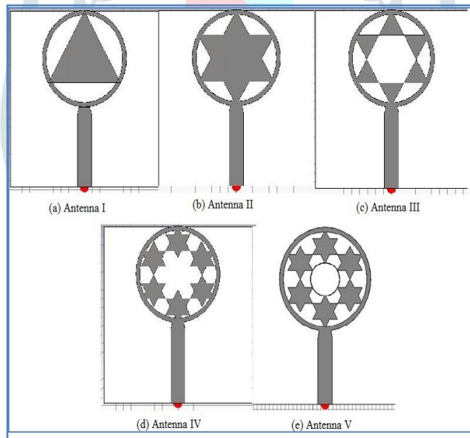
Figure 2: Intermediate steps of designing antenna structure
