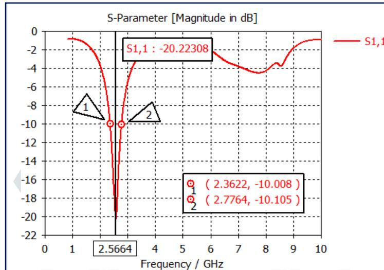
Figure 3: Reflection coefficient of fractal antenna
