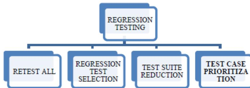
*Figure 1: Regression testing approaches*
