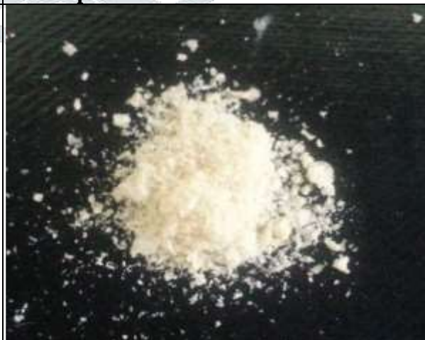
Fig. Pre-treatment of chicken feather with petroleum ether for 24 hours.
