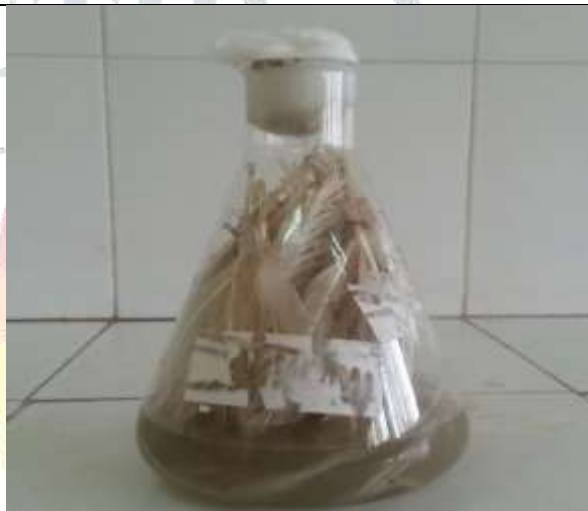
Fig. Pre-treatment of chicken feather with petroleum ether for 24 hours.
