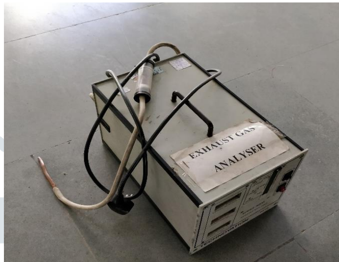
Fig. 3.2 Exhaust gas Analyzer
