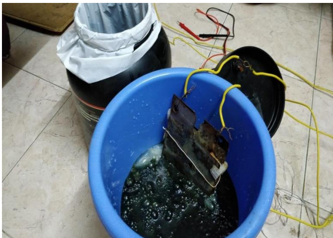
Fig. 2.1. Electrolysis with NaCl as electrolyte
