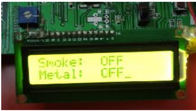
Fig 3(a) Smoke and Metal not detected
