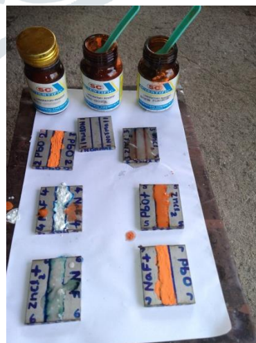
Fig 3.3. Flux Coating over Steel Plates
