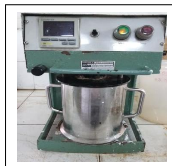
Fig.- 3: Disintegrator used for pulping purpose
