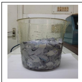
Fig.-2: Soaking of small size papers
