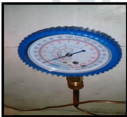
Fig.11 Attaching suction & delivery pressure gauges
