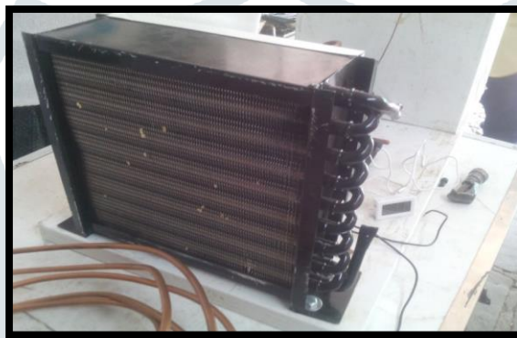
Fig.10 Fixing Condensor on platform
