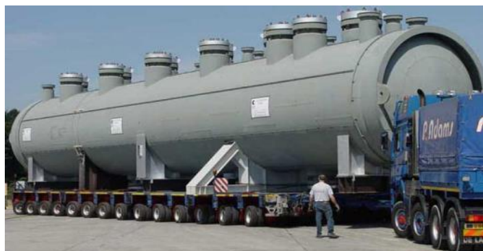
Figure 6 (a) Titanium Clad pressure vessel (Picture is the property of Coek Engineering NV, Lessel 13-2440, Belgium)
