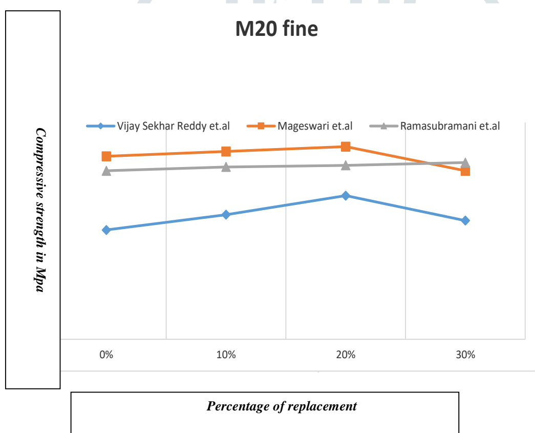
Fig 1: Comparison of compressive strength between different authors for replacement of fine aggregate with WG for M20 grade.
