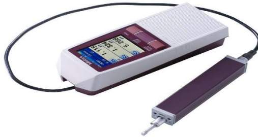
Fig.4 - Surface roughness tester [12]
